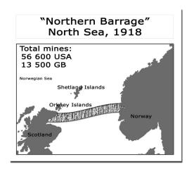
Norway would be required in order to 'close' the northern outlet of the North Sea, 150 sea miles (approx. 275 km). Near the Norwegian coast, the water is 300 metres deep and near Orkney, about 100 metres. Sea currents can reach 3-4 nautical miles/hour. That was a challenge which required the development of a new mine, the MK6. The charge consisted of 300 pounds of grade B trinitro-
